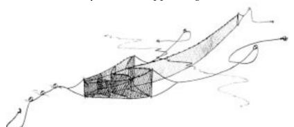
Figure 1. Fyke net.
